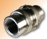
The **SNS** is an ideal solution for the production power unit builder. Weld the SNS below fluid level to your reservoir. An internal thread or Sch.40 socket allows mounting of strainer or baffle pipe. External SAE/ISO/BSP swivel thread permits perfect alignment of shutoff valve — it's a win-win solution for speed and quality.
