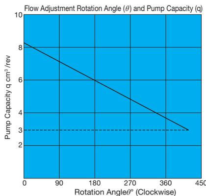
The values indicated above are at maximum pump discharge volume with the flow volume adjusting screw at the 0° position.
